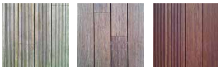
Surface of MOSO® Bamboo X-treme® with different maintenance and cleaning scenarios: weathered, dirty decking (left), weathered, cleaned decking (middle), and re-oiled decking (right).
